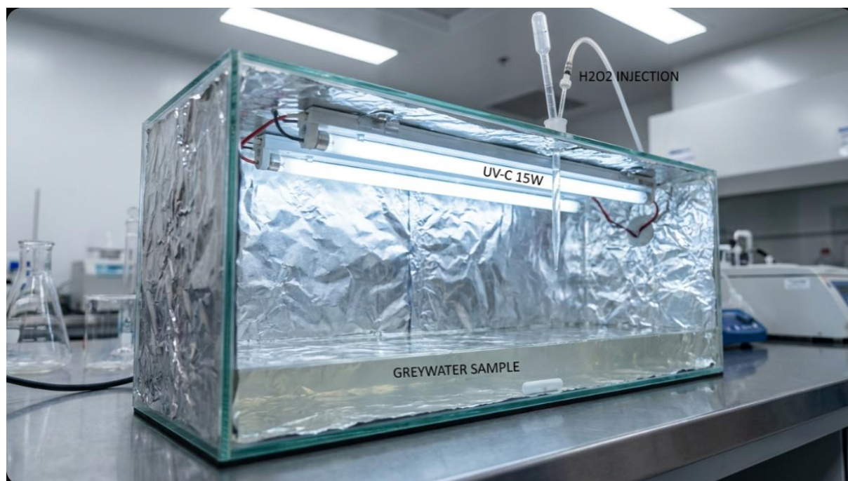
Figure 1. Schematic diagram and component identification of the UV/H 2 O 2 photo-oxidation pre-treatment system.
