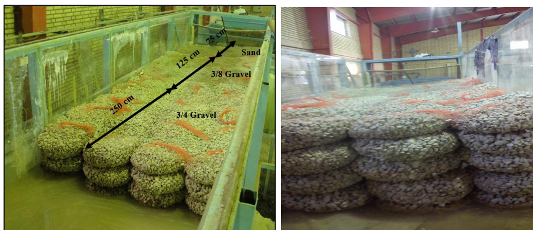
Figure 3- Filter layout in the laboratory flume
