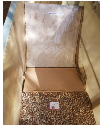
Figure 2-Spillway of a flip bucket and riprap at the downstream
