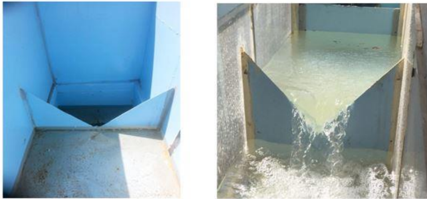
Figure 2- Triangular inlet and outlet overflows with 90-degree vertices, at the beginning and end of the flume.
